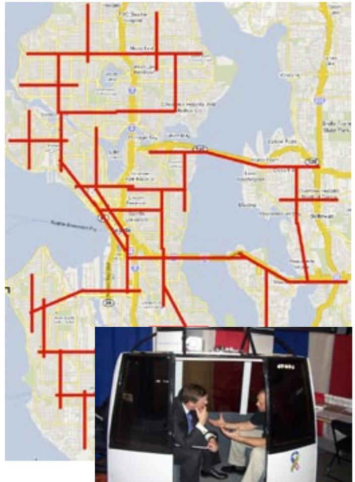
**Rescue-Rail:** Rescue-Rail is a temporary version of Intelligent Transportation and ET3. These are deployed on temporary basis for a limited time in response to a specific emergency or special event. The objective is to deploy 30 to 60 miles per day per installation team. This rate of deployment requires routes to be pre-surveyed and pre-planned for deployment. Routes may require access to road and or rail right of ways.
