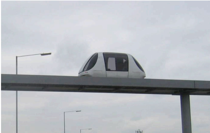
Figure 3 ULTra Vehicle on Elevated Track
