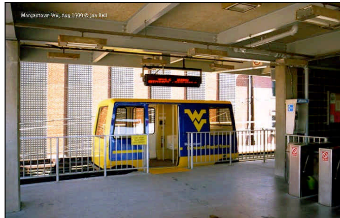
Figure 4: Protective Safety Fence. Courtesy of Jon Bell.
