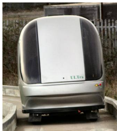
Figure A-4 - ULTra Vehicle On Surface Guideway Image Courtesy of ATS
