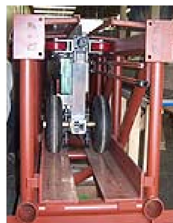
Figure A-2 - Skyweb Express Bogie Inside The Guideway Image Courtesy of Taxi 2000
